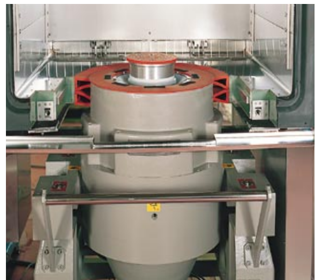
Photo. 9 Vibration generator connected to temperature/humidity chamber
